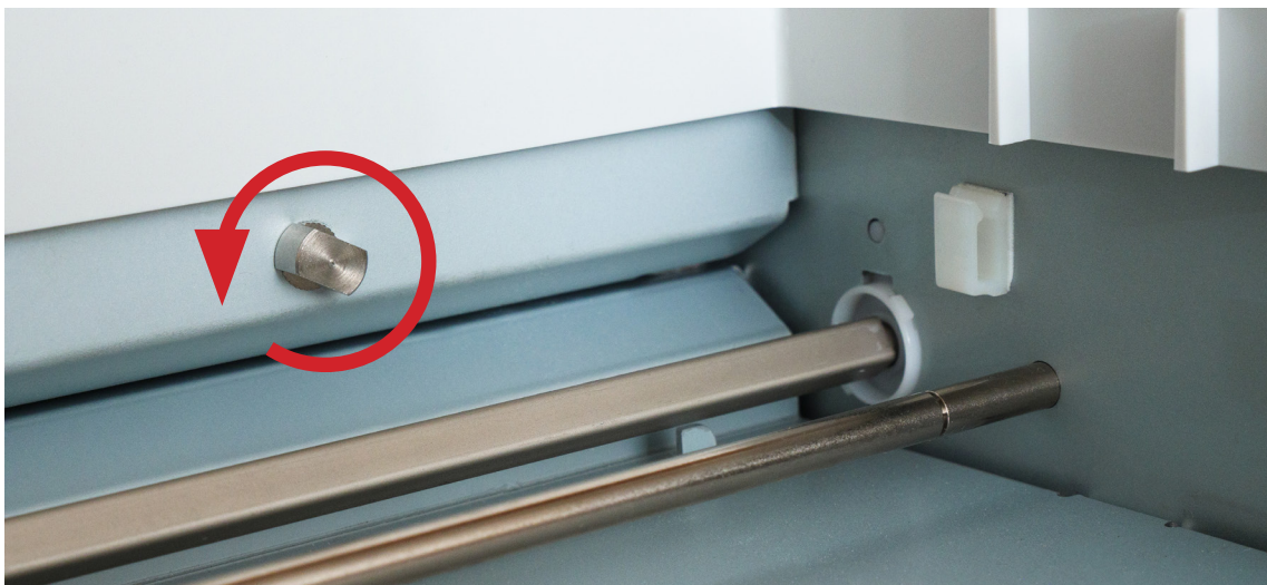
Image 1: Shows the shipping bolt and location
